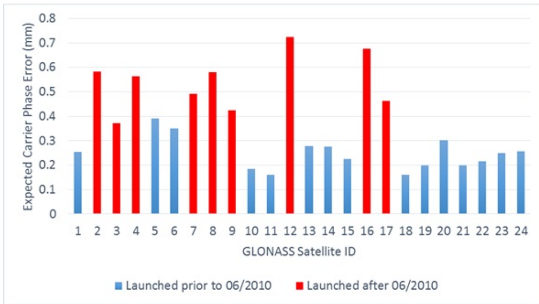
Figure 7.16: Maximum 1-second carrier phase error due to onboard oscillator instabilities for the current GLONASS constellation.
